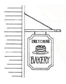
*SIGN, SUSPENDED.* A sign, which is suspended from the underside of a horizontal plane surface, such as a canopy or marquee, and is supported by such surface.
